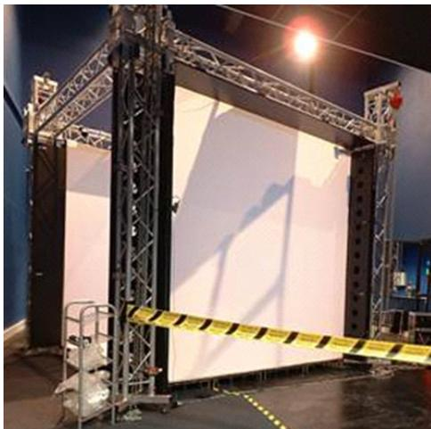
Figure 1: A Immersive Display: The SAS-CUBE<sup>TM</sup>
